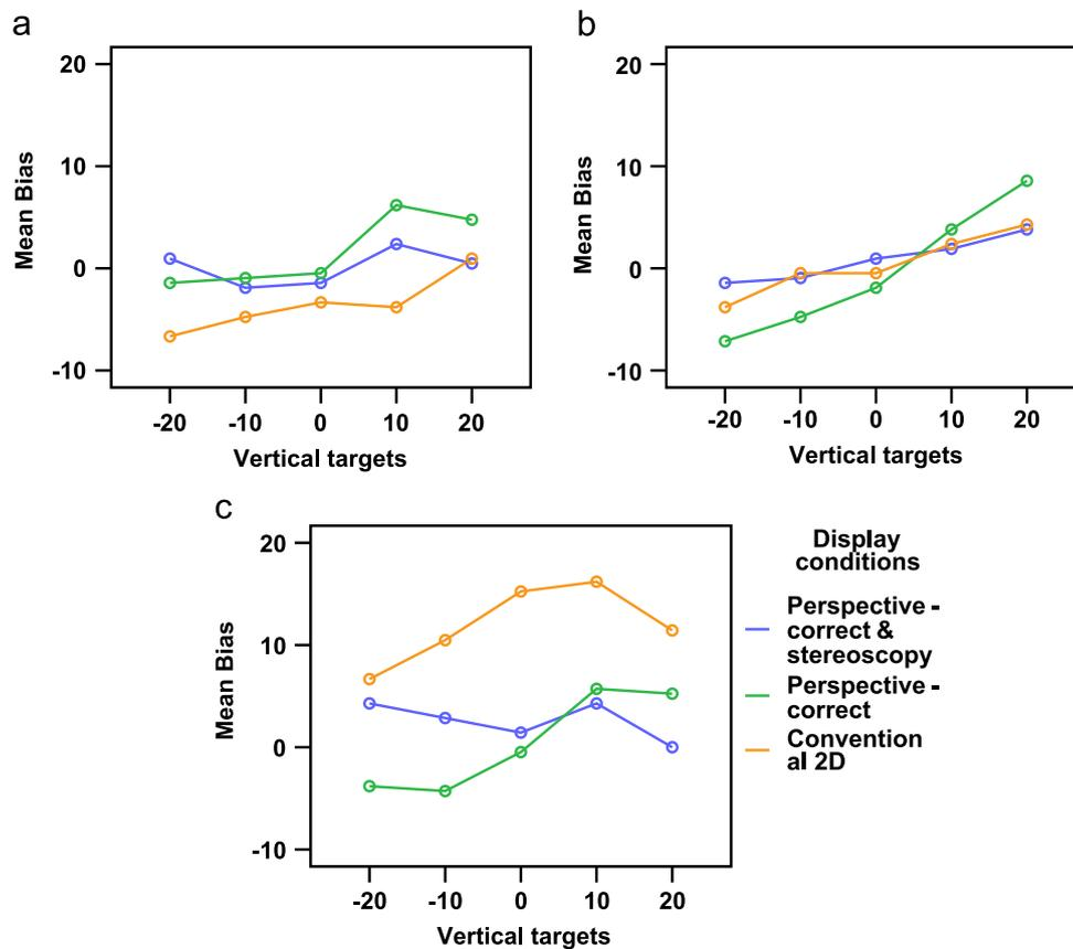
**Fig. 13.** The mean vertical bias for each display conditions, vertical viewing angles and horizontal target position. (a) Vertical viewing angle  $-10^\circ$  (b) Vertical viewing angle  $0^\circ$  (c) Vertical viewing angle  $20^\circ$ .
