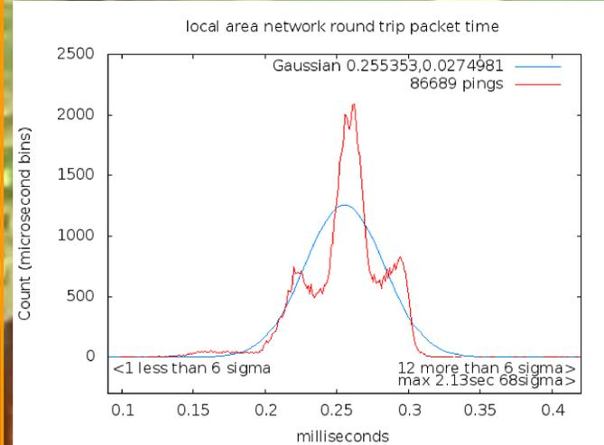
Figure 3: Distribution of network delays over one day. Notice approximately Normal distribution but very long tails (especially long delays).
