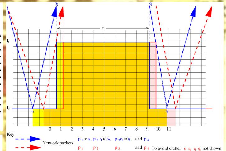
Figure 4: Start and stop network messages (arrows) are used in distributed energy measurement. Network jitter means two measurements of same software give different answers (yellow and pink). Fast LAN and 12 bit 1KHz ADC quantisation noise dominates jitter.
