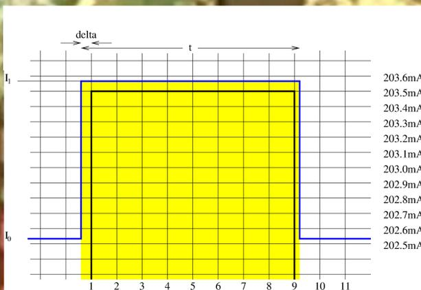
Figure 3: Energy used is area under curve (yellow) but only area inside quantised rectangles is recorded. E.g. noise = 7%
