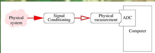
Figure 1: Physical measurement (e.g. thermocouple, resistor) converts signal to voltage, which ADC converts to number (e.g. 0 to 4095).
