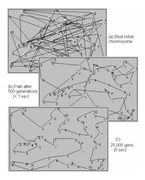
**Figure 2** TSP problem. (a) Best random path (chromosome) from initial population (b) Best path after 500 generations (c) Best path after evolution through 25,000 generations (only 6 seconds of evolution for this simple case).
