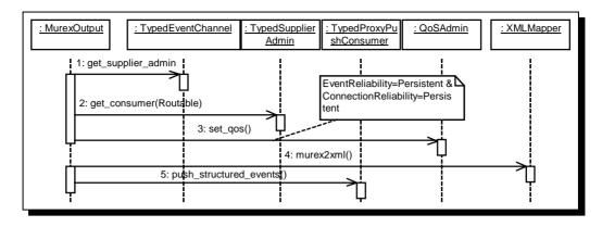
Figure 5. Output Adapter Interacting with Notification Service
