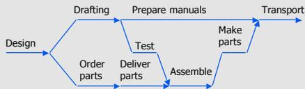
shows operations required to produce custom made machine
