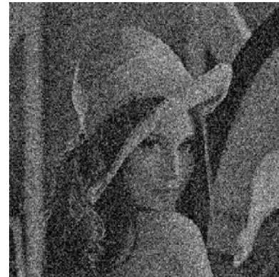
Figure 5.11 Watermarked image after Gaussian attack
