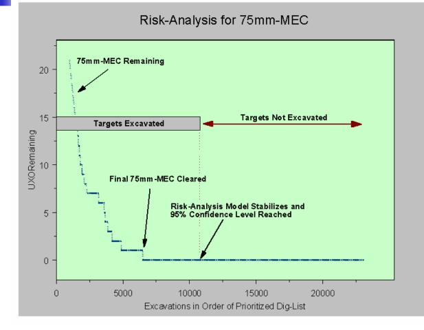
Note: Excavation continues even after the final 75mm in cleared until the predetermined confidence (stopping) criteria is reached.
