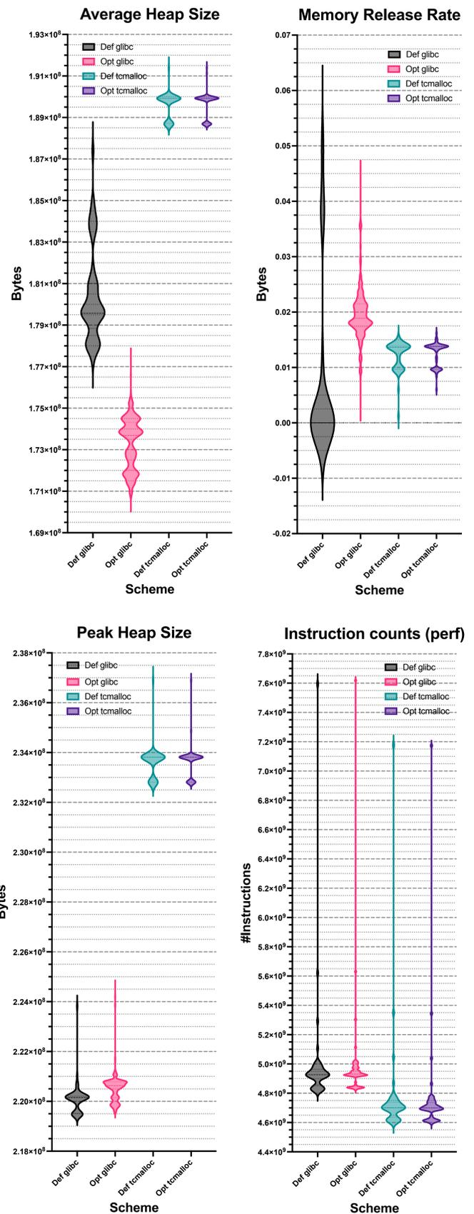
Allocator trade-offs differ: glibc allows gradual tuning with small changes in instructions and heap, while TCMalloc operates near optimal boundaries, offering higher peak-heap potential but requiring steeper trade-offs.
