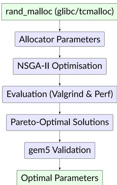
We begin with rand\_malloc, a lightweight benchmark emulating gem5's memory behaviour. Allocators (glibc and tcmalloc) are configured, and a multi-objective genetic algorithm (NSGA-II via pymoo) optimises both peak heap usage and instruction count. The resulting Pareto-optimal configurations are then validated on gem5 to identify the best-performing parameters.
