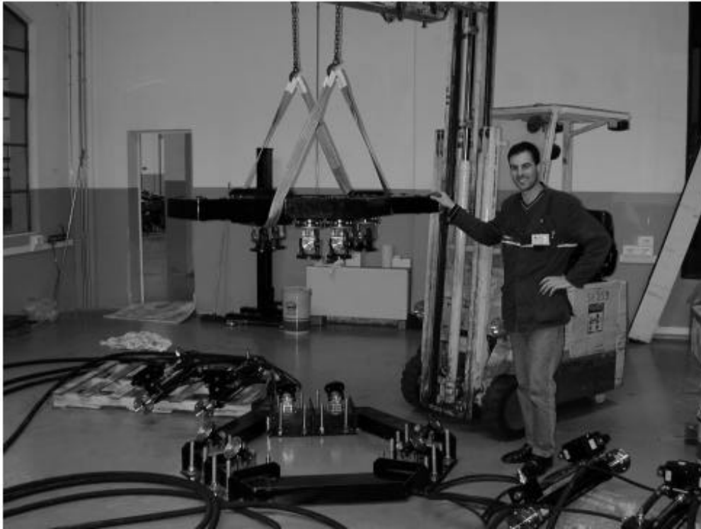
Figure 6-5 Final SP Manipulator during mounting phase
