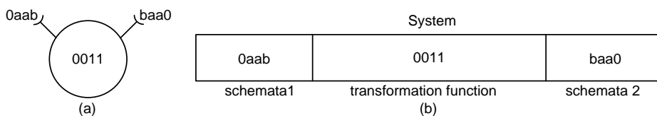
Fig. 1. SC notation and systems representation: a) Graphical representation of a system in SC. b) The three elements of a system. (Reproduced with permission from [1]).
