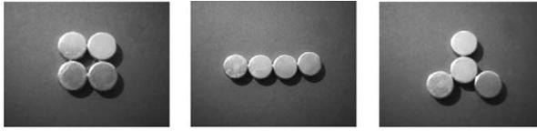
FIG. 7. The three stable two-dimensional formations of magnetic discs: grid (left); chain (centre); and triangular (right).
