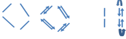
Figure 5. Graph construction as in [17, 30]: Left: A bidirected graph is constructed by separately treating edges with different directions. Right: Connections among conjugate nodes help detect open contours as cycles in a graph.
