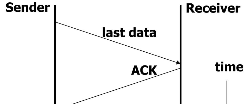
**Risk:** new connection opened; delayed data from old connection arrive at receiver during new one
