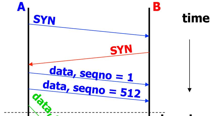
**Connections shouldn't start with constant sequence number; risks mixing data between old and new connections**
