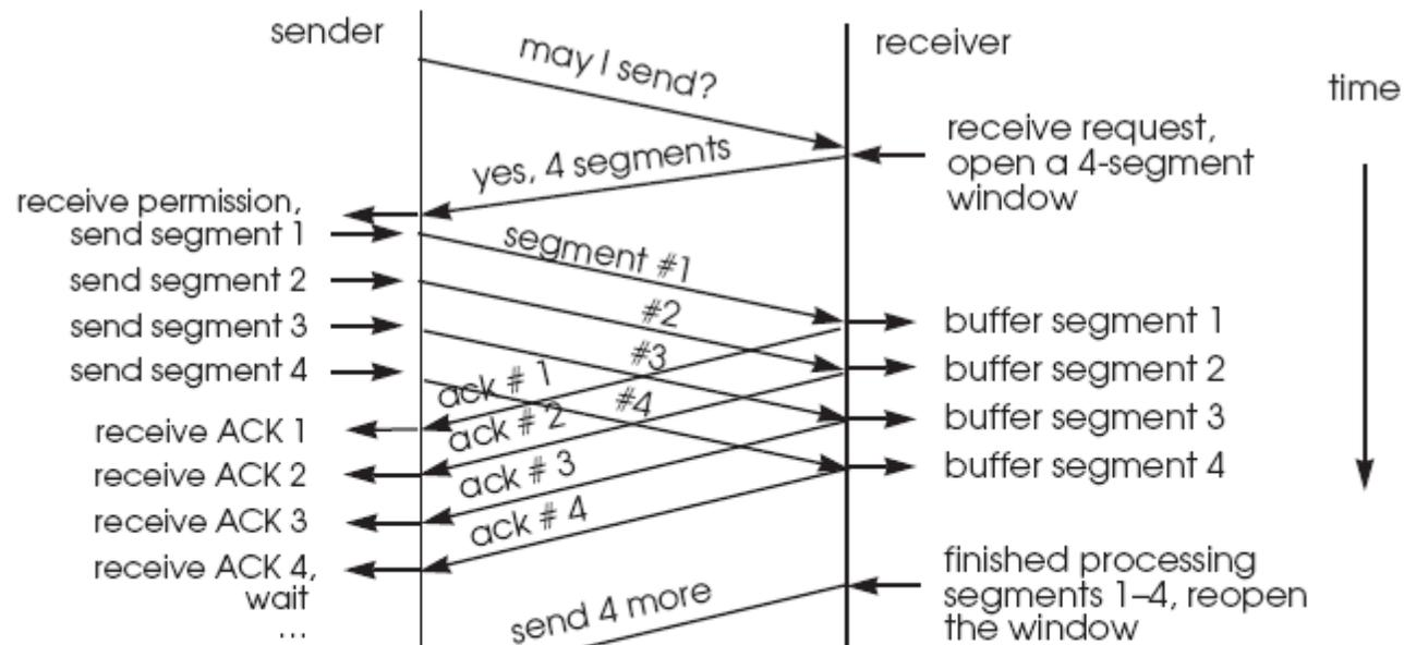
**1 RTT idle time between grant of new window and arrival of data at receiver**
