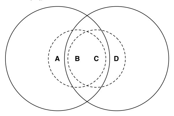
Nodes A and D in the figure transmit with high power, while nodes B and C transmit with low power. There are four circles drawn in the figure. Each circle represents the transmit range of the node on which it is centered. The solid circles represent the transmit range of nodes A and D, while the dashed circles represent the transmit range of nodes B and C.
