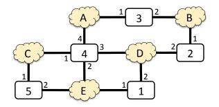
Here clouds labeled with letters represent LANs, and each bridge (also known as a switch) is numbered with its identifier. The numbers just outside each switch in the figure above are port identifiers.
