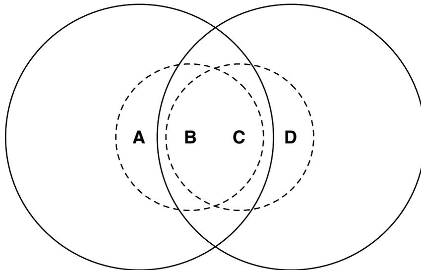
Nodes *A* and *D* in the figure transmit with high power, while nodes *B* and *C* transmit with low power. There are four circles drawn in the figure. Each circle represents the **transmit** range of the node on which it is centered. The solid circles represent the transmit range of nodes *A* and *D*, while the dashed circles represent the transmit range of nodes *B* and *C*.
