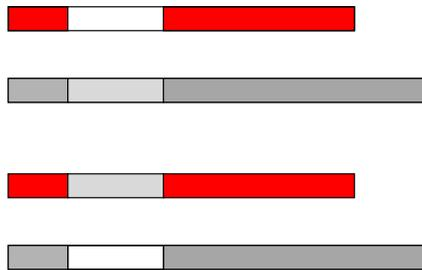
**Figure 4.** HXO crossover. As with the other crossover operations, two parents (top two programs) crossover to yield two child programs (bottom). In HXO the two crossover cut points are the same in both parents. Note code does not change its position relative to the start of the program (left edge) and the child programs are the same lengths as their parents.
