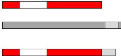
**Figure 3.** XOA crossover. If there is no length overlap between code selected in second parent and the first parent (top), the selected code fragment is appended to the whole of the code from the first parent. (I.e. the middle portion of the first parent is not removed.)
