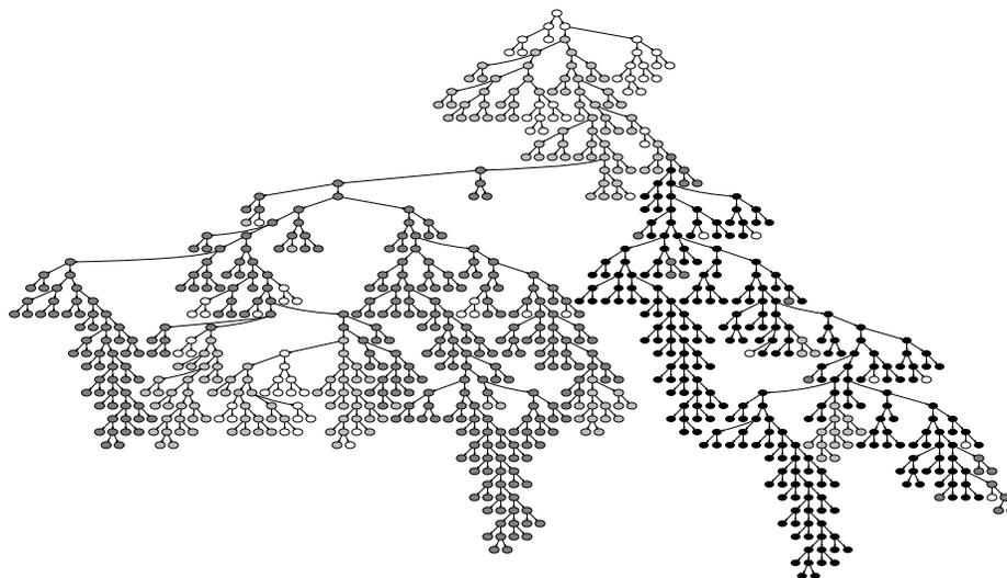
**Fig. 5.** Repeated patterns in the largest protein prediction program (2XO, 843 nodes). largest pattern (133 nodes) in black. Other nodes in repeated patterns are filled according to size of the repeated pattern (33–132 grey and 11–32 light grey). Unique nodes and nodes which are part of small patterns are not filled.
