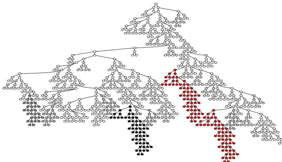
**Fig. 6.** Same program as in Figure 5. Here whole subtrees are exactly repeated. Nodes are filled according to size of the repeated subtree. Unique nodes and nodes which are part of small patterns (3 nodes or less) are not filled. Two largest (59 nodes, right hand side) coloured red. Note these are partially repeated elsewhere in the tree (e.g. 55 node subtree shaded black).
