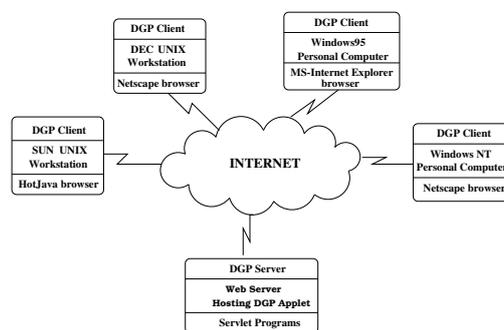
Figure 1: Four workstations of different types work asynchronously over the Internet on a common GP problem using a distributed population, communicating occasionally via Servlet programs.
