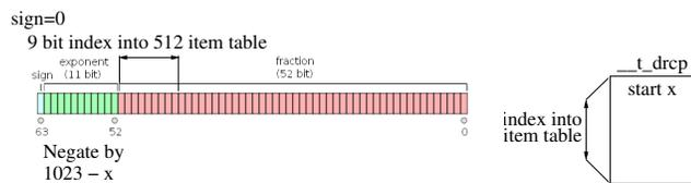
Figure 6: GI `drpc`. Left: to negate the exponent of positive double (11 bit two's complement integer), `drpc` subtracts it from 1023. `drpc` uses the top 9 bits of fractional (mantissa) part give a nine bit index. Right: index used with float `__t_drpc` of initial values for Newton-Raphson iterative solution of  $\frac{1}{x}$ .
