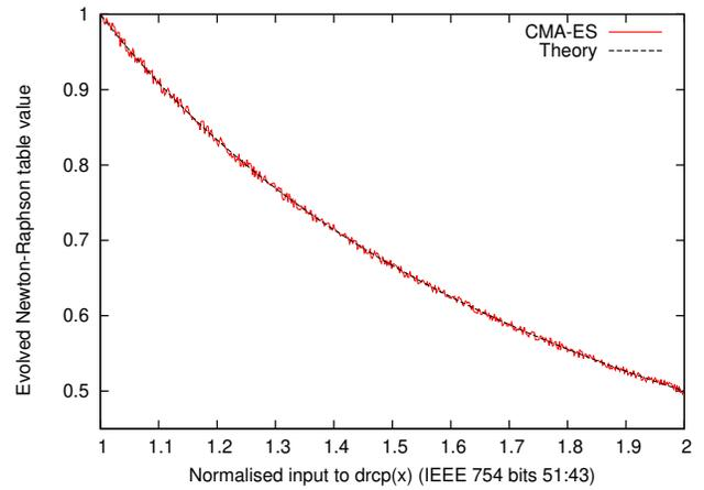
**Figure 10: 512 GI table values for  $\text{drcp } x^{-1}$ . They are shown plotted against normalised  $x$  input to  $1/x$  (horizontal axis), and corresponding  $\text{inv}$  table value (vertical axis).**
