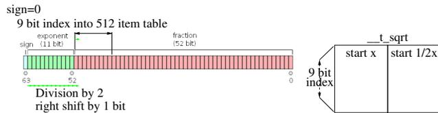
Figure 5: Left: `e_sqrt.c` uses right shift of exponent of positive double (bit 63 = 0) to a) divide exponent by two and b) merge least significant bit with top 8 bits of fractional (mantissa) part to give nine bit index. Right: index used with float `__t_table` containing 512  $x_1$  and  $1/2x_1$  pairs of initial values for Newton-Raphson iterative solution of  $\sqrt{x}$ .
