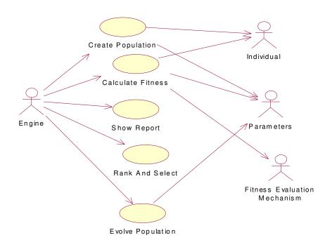
Looking at a higher level, a use case diagram can be used to show what the user is able to do, and what engines and parameters need to be accessed to achieve these choices.
