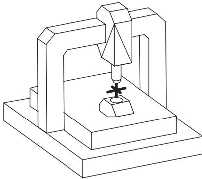
**Figure 2. A typical coordinate measuring machine**
