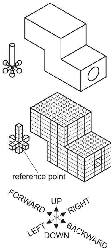
**Figure 3. Discretization of the part and the probe**
