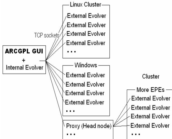
**Figure 3.** External parallel evolver architecture.
