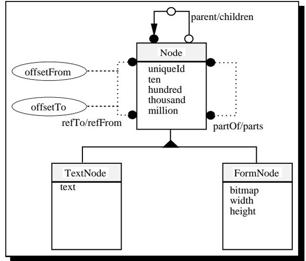
Figure 2: Conceptual schema of the Hypermodel benchmark
