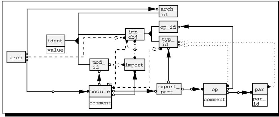
Figure 6: EER Diagram of simplified Database Base Schema
