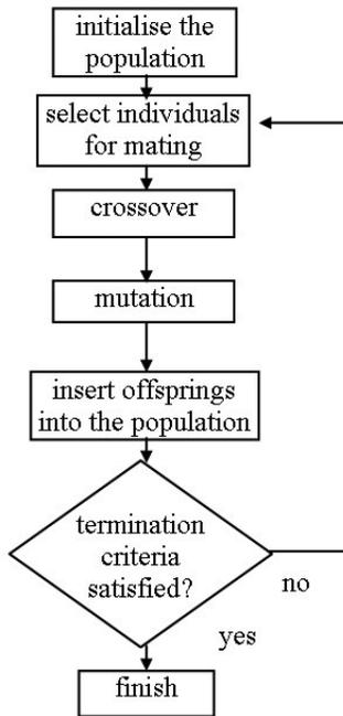
FIGURE 2. Flowchart for a basic GA.
