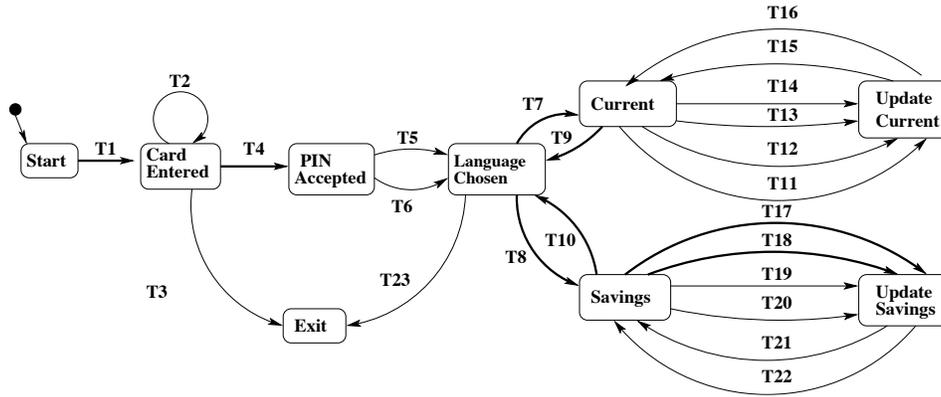
Fig. 9. The slice generated for the ATM system (shown in Figure 5) with respect to  $(sb, T18)$  using Labbé and Gallois [2008]. The highlighted transitions indicate the transitions in the slice. The transition labels are given in Table II.
