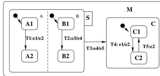
Fig. 4. A hierarchical and concurrent state machine.
