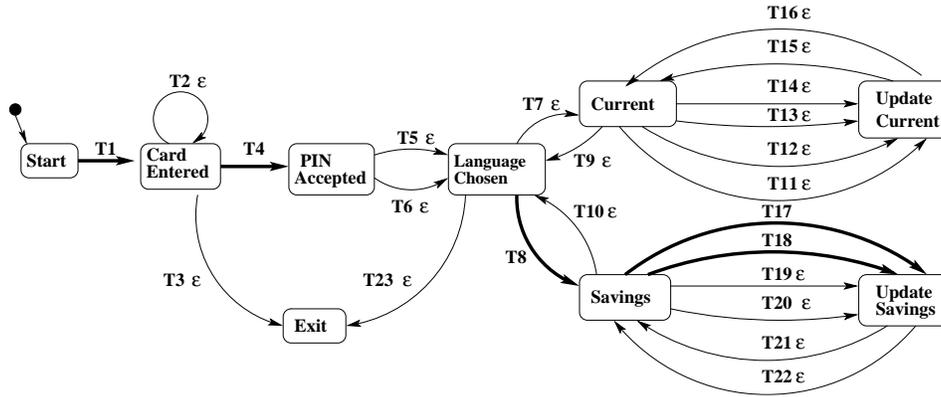
Fig. 8. The slice generated for the ATM system, shown in Figure 5, with respect to  $(sb, T18)$  using the algorithm by [Androustopoulos<sup>†</sup> et al. 2009]. The labels of marked transitions (highlighted) are given in Table II, while unmarked transition have the label  $\varepsilon$  indicating an empty label.
