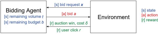
Figure 1: Diagram of reinforcement learning to bid.
