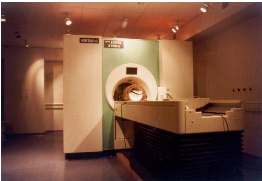
Figure 1.1: The 3T Varian/Siemens magnetic resonance imaging system installed at the Oxford Centre for Functional Magnetic Resonance Imaging of the Brain (FMRIB) where the research described in this report was carried out. It is designed specifically for ultra-fast imaging in brain functional magnetic resonance imaging studies and is equipped with both a body gradient coil and a fast head gradient coil insert.
