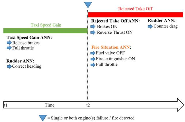
Fig. 7. (Rejected Take Off experiment) The behaviour of the IAS when engine(s) failure or fire is detected and a Rejected Take Off (RTO) is performed. The Fire Situation ANN is used only when fire is detected.
