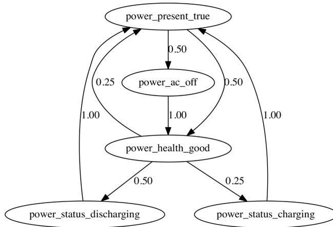
Fig. 5: Markov chain for the battery status.
