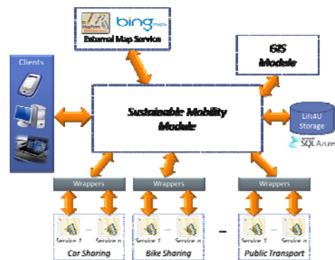
Figure 1: The modules involved in a trip based only on external mobility solutions
