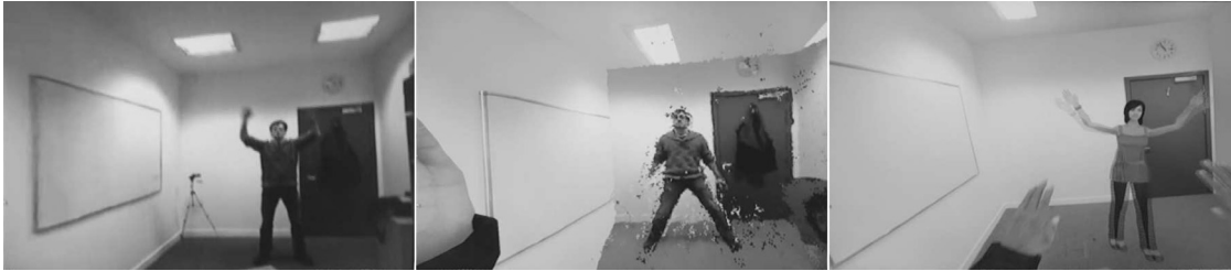
Figure 2. The three display modes available at the visitor site from left to right: spherical video from the Ladybug 3, a hybrid approach featuring embedded 2.5D Kinect video of the destination actor within a VE, and a pure VE featuring Kinect-tracked embodied avatars.
