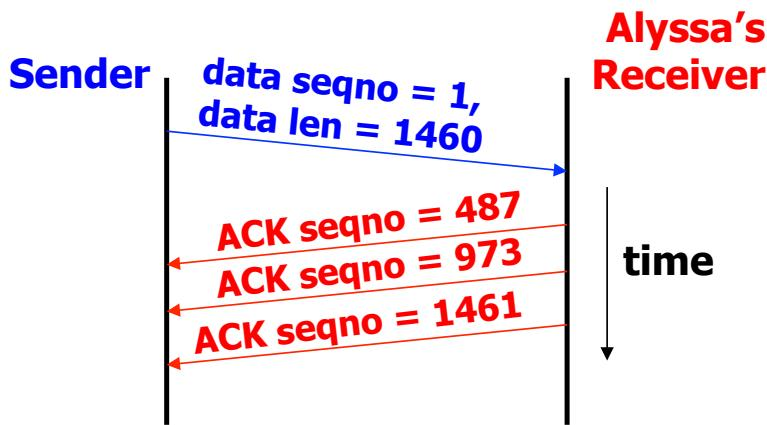
(In the diagram, Alyssa's TCP receiver sends the three TCP ACKs shown back-to-back in time, one immediately after the other.)
