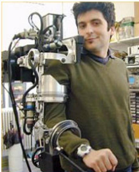
Figure 2: *Haptic Interface developed by PERCRO at Scuola Superiore S. Anna, Pisa, Italy*
