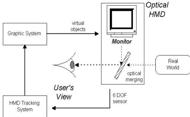
Figure 3: AR system using the optical see-through HMD.
