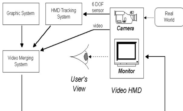
Figure 4: AR system using the video see-through HMD.
