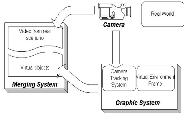
Figure 2: AR system with tracked camera.
