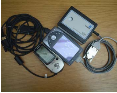
Figure 1 Early prototype of the mobile pollution-logging device
