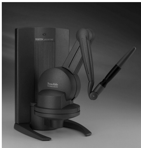
Figure 1. While users held the pen-like stylus (on the right) performing writing-like movements, the attached force-feedback mechanism generated a resisting force—haptic stimulation. Users responded by pressing a button on the stylus.
