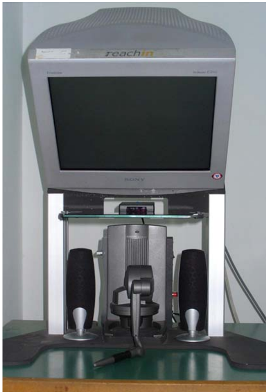
Fig. 1 Experimental setup. The visual display from the computer screen was reflected onto the horizontal mirror. Participants looked at the mirror while holding the pen-like stylus in their hand and positioning it at the center of their visual field. Two loudspeakers were placed in both sides of the stylus. In every trial the computer generated a uni-, bi- or tri-sensory stimulation, randomly, and participants were required to press the corresponding button(s)
