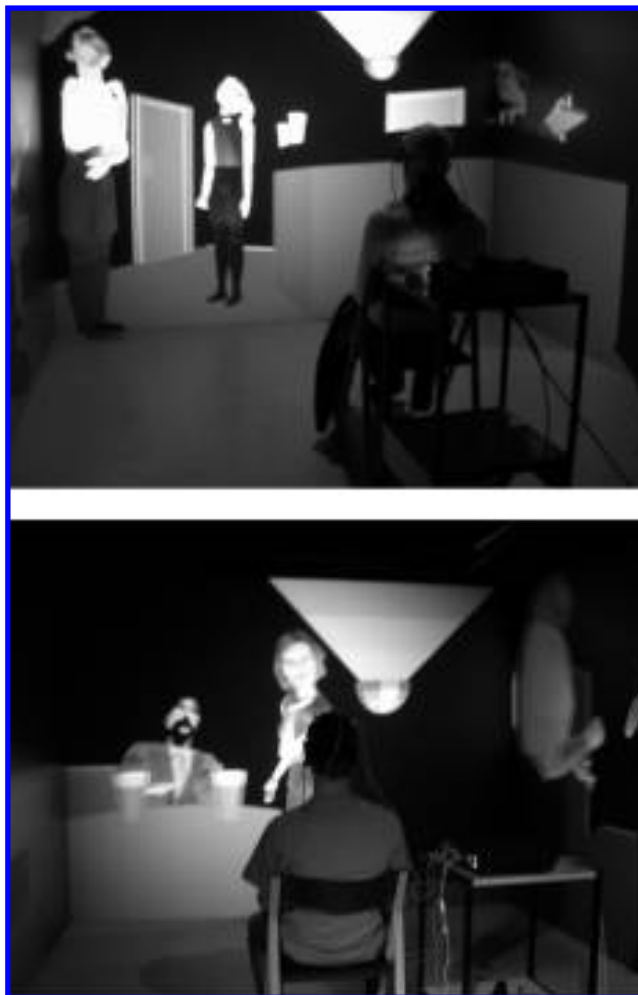
Figure 2. Two images of a subject connected to the BCI, wearing shutter glasses, in the virtual bar VE in the VR CAVE room. Using only his thoughts, the subject can rotate the VE to pay attention to different characters in the bar.
