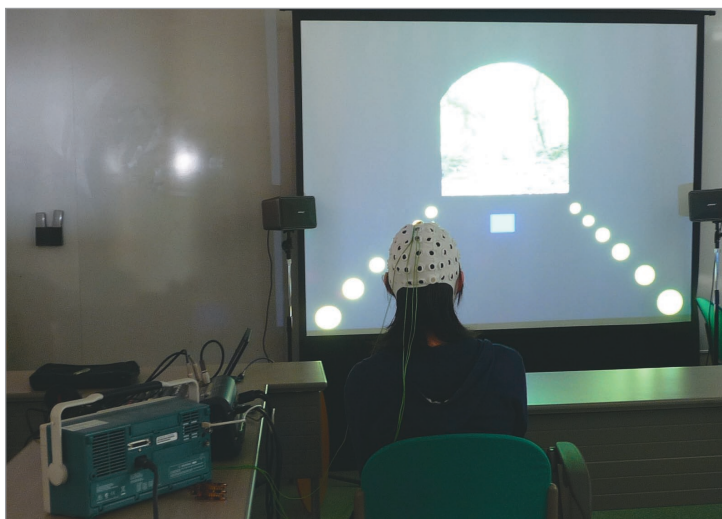
Figure 3. Monitoring drivers' alertness level in a virtual reality driving simulation using BCI and P300 signals.
