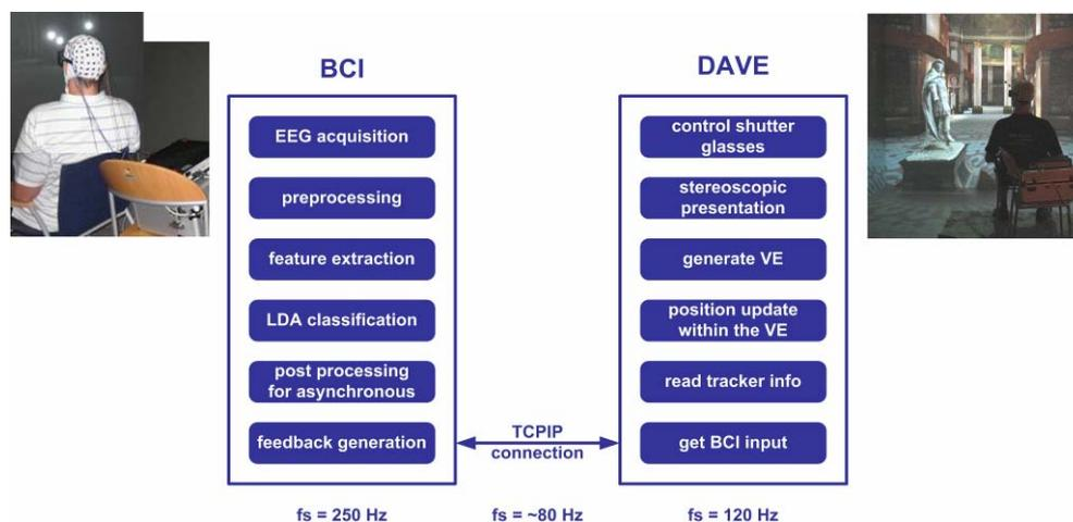
**Figure 1.** System diagram of the hardware setup. The BCI system on the left analyzes the EEG signals and the extracted control commands were transferred into movements with the VE projected in the DAVE system.
