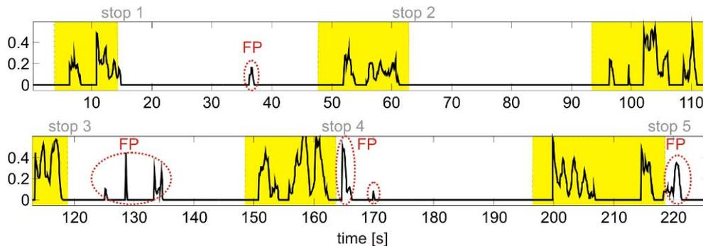
**Figure 6.** Online performance of the first run of subject al10. The yellow rectangles mark the periods when the subject should move to the next point. The black line is the actual BCI output after the postprocessing. Whenever the line is not zero a movement occurred. Periods of FP are indicated with red dotted circles.
