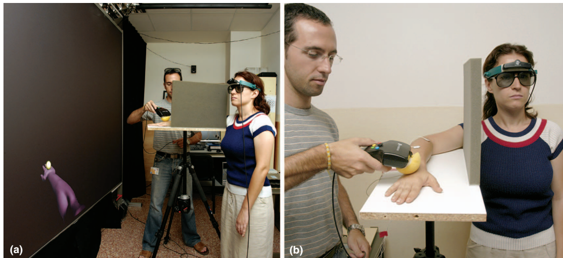
1 Recreating the “rubber arm illusion” experiment. (a) The participant sees a 3D stereo projection of an arm emerging from her right shoulder, with the room otherwise in darkness, while (b) her real arm is hidden. The experimenter uses a tracked wand to stimulate the participant’s real hand while, in synchrony, a virtual ball slaved to the wand strikes the virtual hand. After a few minutes of this, most people feel the virtual arm to be their real arm—a phenomenon demonstrated in both subjective reporting and behavioral and physiological measures.
