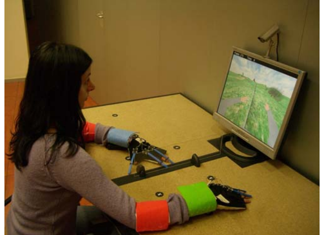
Fig. 1. The Rehabilitation Gaming System setup. The user wears color patches that are tracked by the motion capture system and these are mapped onto a virtual character. Data gloves provide the finger flexion data. The screen displays a first person view of the gaming scenario in the virtual environment. The dots on the table are the reference points during the evaluation phase of the system.
