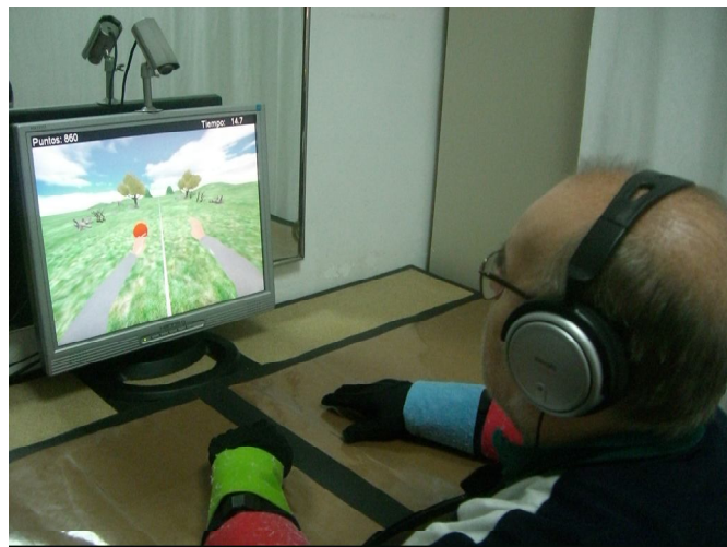
Figure 1. The Rehabilitation Gaming System. A subject faces a display with the arms resting on a table. The arm movements are tracked by a camera positioned on top of the display. The tracking system detects in real-time the position of the color patches located on the wrists and elbows. Data gloves are used to detect finger movements. This way, on the display two virtual arms reproduce the movements of the subject’s arms.
