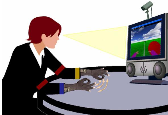
**Figure 1.** The Rehabilitation Gaming System (RGS). The subject, resting the arms on a table surface, faces the computer screen. The movements of the arms are visually captured by a camera positioned on top of the display that detects color patches located on wrists and elbows. A pair of data gloves measure finger flexure. An avatar moving according to the movements of the user performs a task in the virtual scenario. Adapted from Cameirão et al. [46].
