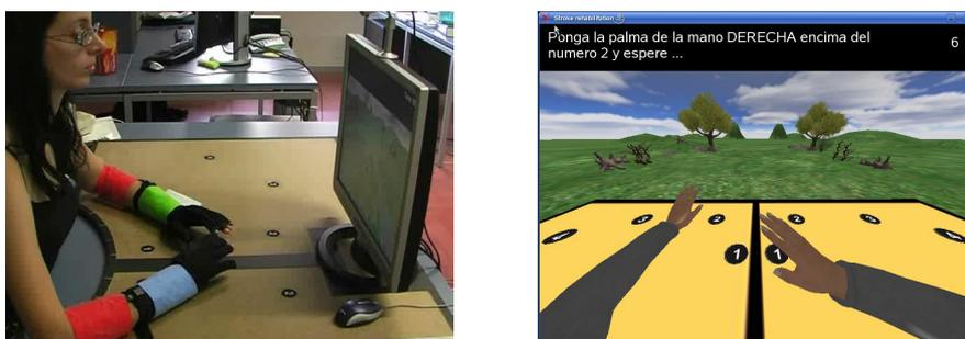
**Figure 2.** Real and virtual calibration phases. Left panel: on the table surface, numbered dots are located at specific positions on the left and right hand sides. The user is asked to place the palm of his/her hand on the numbered dots in a randomized order. Right panel: the same setup is replicated in the virtual environment and the user is asked to perform the same task with the virtual arms. The figure text reads “Place your right hand palm above the number 2 and wait...”.
