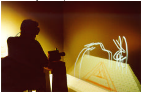
Figure 5. Subject in UCL CAVE, normal-scale/stereo/head-tracked mode (joystick is not in use and is tilted out of the way).
