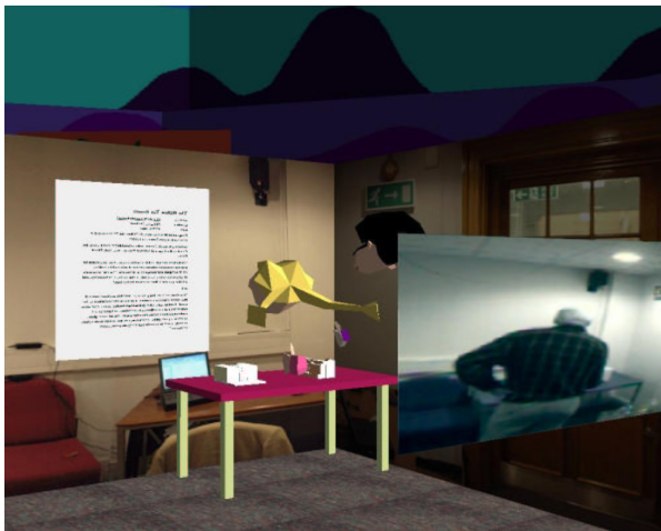
Figure 4 Third person view looking at the two-way boundary view back into the real space with the VE model of the real space. The avatars of the real user and the IPT user can both be seen facing a table.
