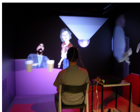
Figure 2: Two images of a subject connected to the BCI, wearing shutter glasses, in the virtual bar VE in the VR Cave room. Using only his thoughts, the subject can rotate the VE to pay attention to different characters in the bar.
